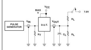
Test Circuit for 3-State Outputs on A Port
